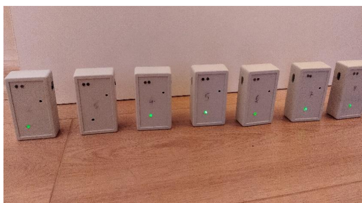
Figure 4.3. Sensor configuration such that gravitational effect on the y -axis
